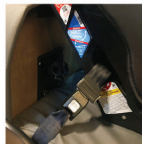
RUN LAP BELT THROUGH BACK OF CAR SEAT AND SECURE. TIGHTEN AS NEEDED.
